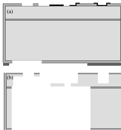
Figure 3. Fabrication schematic for 3-level SCS structures. Four masks, two on front- and two on back-side are done first, and followed by back- and front-side silicon etches.
